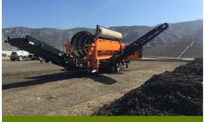
A trommel is used to screen finished compost product into different particle sizes.
