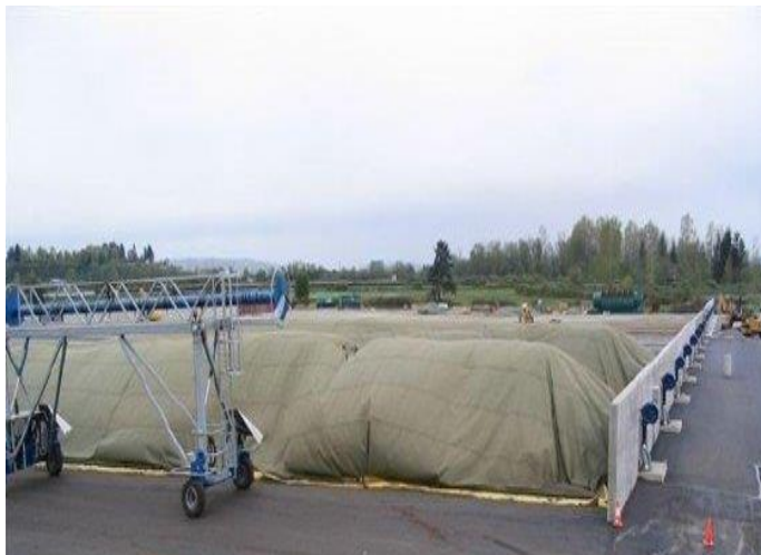
Covered Aerated Static Piles
